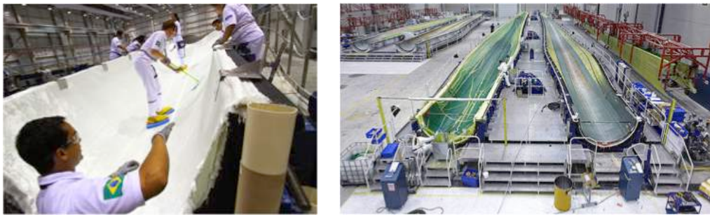
Figure 2. Surface textile material application over the in-mould coating (left) [3]; and resin infusion process of a wind turbine blade [2]
