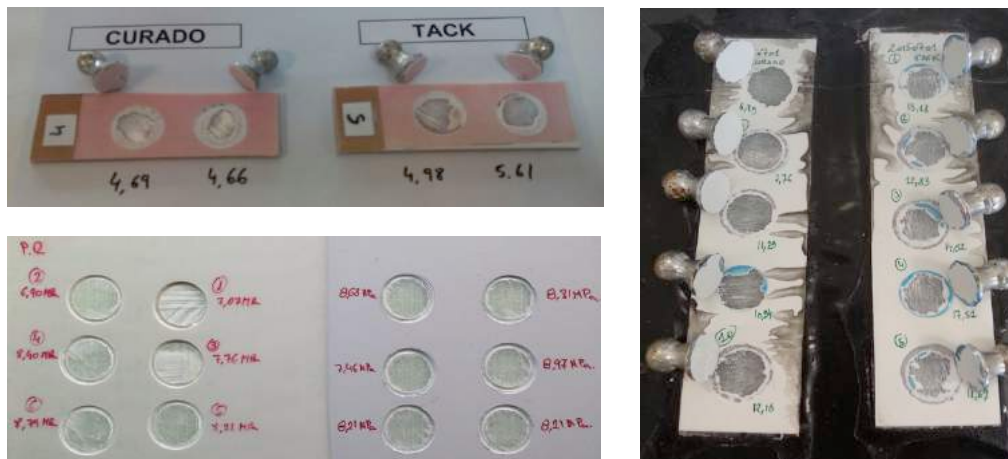
Figure 5. Pull-off strength testing of composite laminates used for coating adhesion (left). Images of the failure in the laminate (right).
