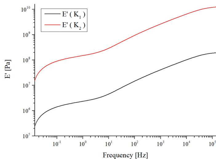
Figure 2 Storage Young modulus obtained with the DMB model for 70 °C.
