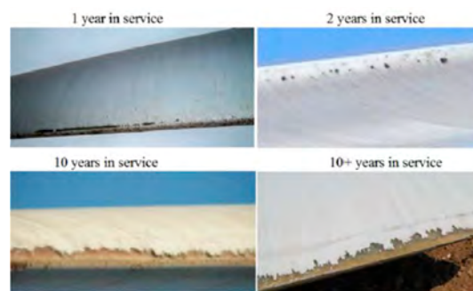
Figure 1. Examples of leading edge erosion across a range of years in service, from [1].
