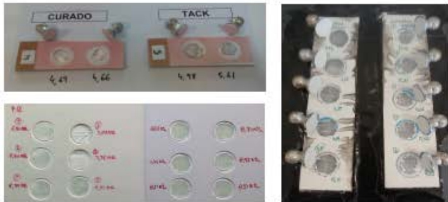
Figure 3: Pull-off strength testing of composite laminates used for coating adhesion show the failure in the laminate
