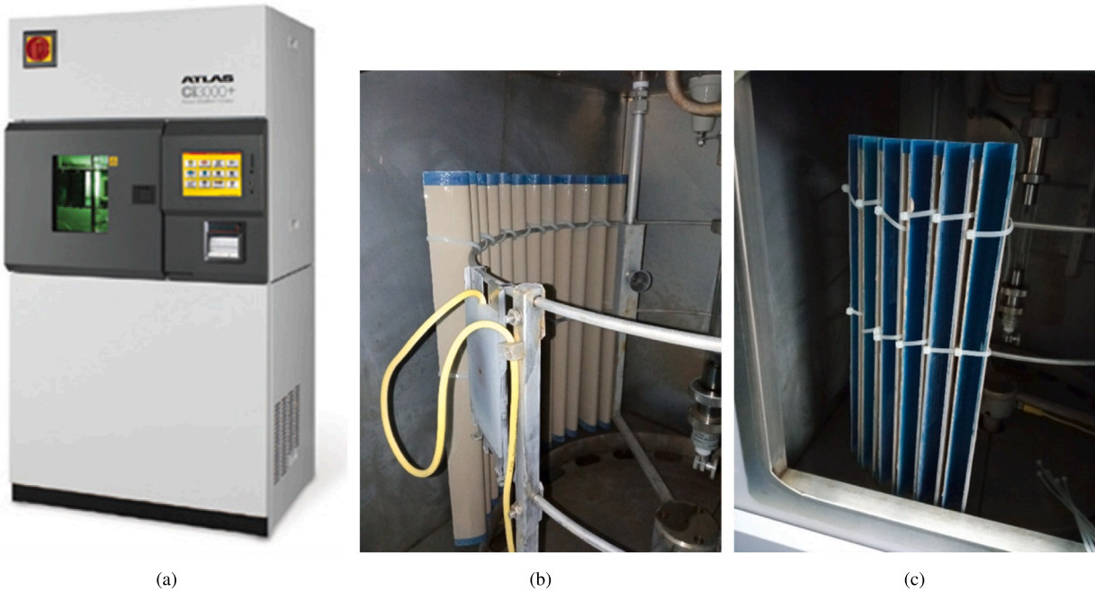
Fig. 5. Hardware for ISO 4892-2 aging of the specimens before RET.
