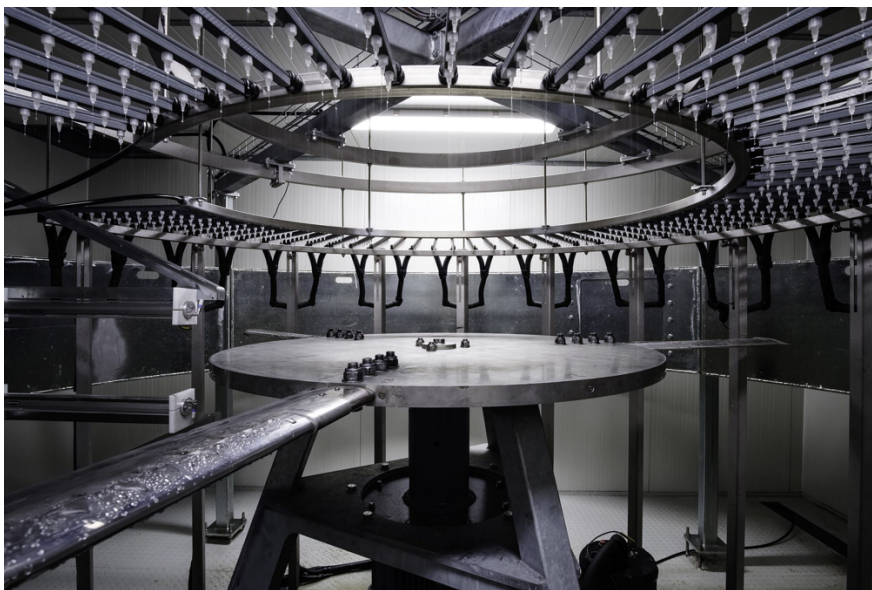
395 Figure 13. Rain Erosion Test developed in Aeronordic, from [32].
